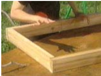
Screw the corners of the frame together
