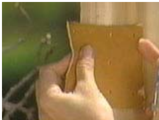
Cut a piece of leather in the shape of a hinge
