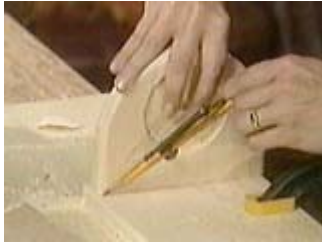
Use the cut off piece to mark for cutting
