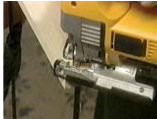
Cut along the lines with a jig saw
