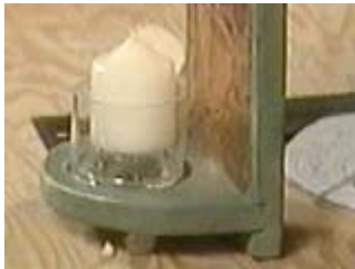
Use a saw and chisel to make a one quarter inch deep groove
