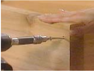
Pre-drill and screw the frame together
