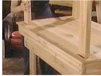
Line the legs up over the holes and drop into position
