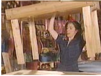
Set the top section in place over the bottom section
