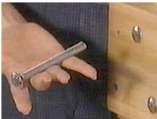
Attach the legs with carriage bolts
