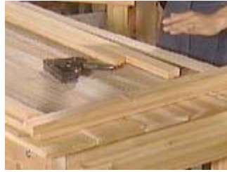
The second half of the frame is attached over the wire and front is screwed to the back
