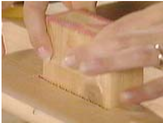
.....and test it with the scrap piece of 2 x 4
