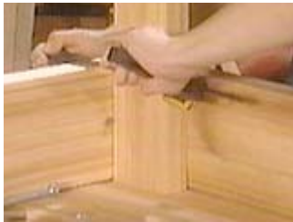
Clamp the leg in place before drilling
