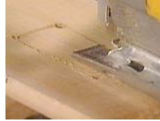
Cut out the hole for the leg...
