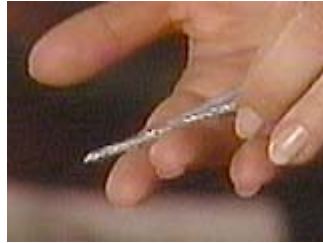
Use galvanized nails with a spiral shank
