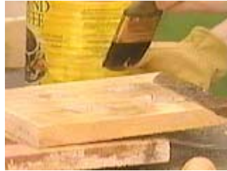
Brush on the stain before attaching the sides together
