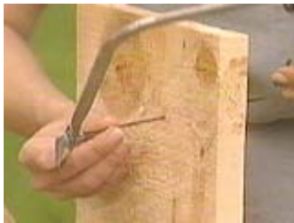
Pass the coping saw blade through the first hole, then reassemble the saw in position
