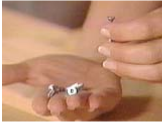
Use zinc or other weather resistant screws.
