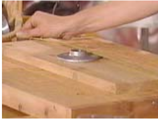
Center the flange on the bottom of the feeder.
