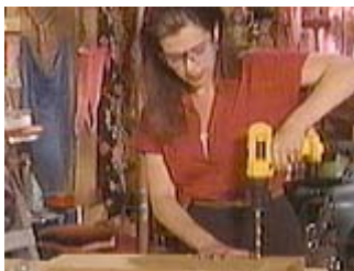
Drill 4, half-inch holes - one in each corner.
