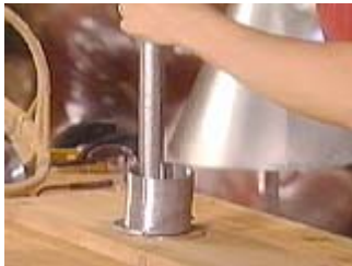
Screw the three quarter inch pipe into the flange.
