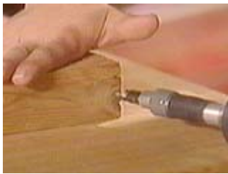
Pre-drill before attaching the sides or ends.
