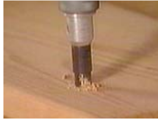
Be sure to countersink for the head of the screw to prevent splitting.
