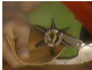
Use a leather punch to make holes for the screws
