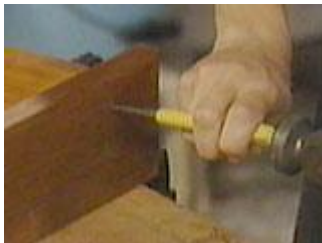
Use a hammer and nailset to sink the nail head below the surface of the wood
