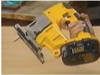
Jigsaw with scrolling blade
