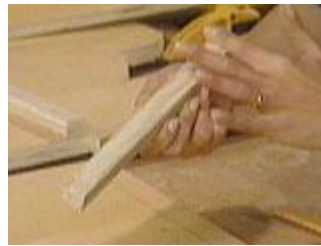
Glue a strip to the back as well
