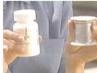
Use flux and leaded solder from a stained glass shop
