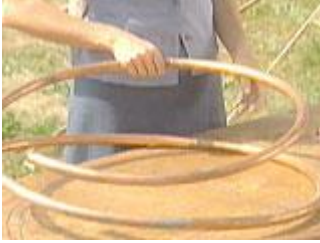
Flexible three-quarter inch copper tubing
