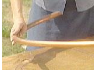
Bend the flexible three-quarter inch tubing to fit the drawing
