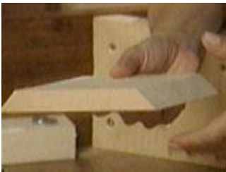
Cut four corner braces with mitered ends
