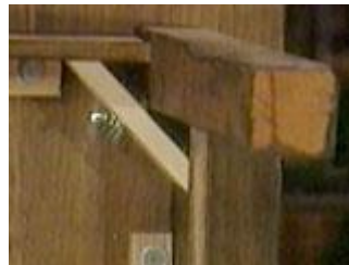
Leg, corner bracket and apron in place
