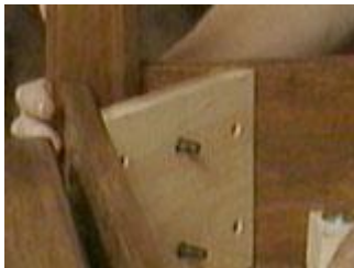
Set the leg in place with the hanger bolts passing through the corner brace
