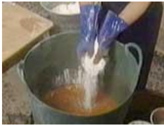
Always add the plaster to the water sifting it through your hands
