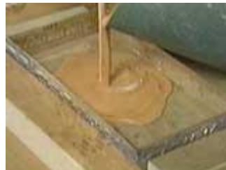
Pour the plaster down a stick to reduce bubbles
