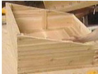
Cut the side piece and install it with screws
