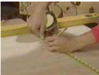
Mark out two 38 inch by 24 inch rectangles
