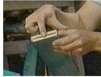
Slot made for the biscuit in the end of an apron piece
