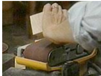
Ease the sharp edges last
