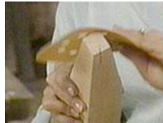
Complete the sanding by hand as necessary
