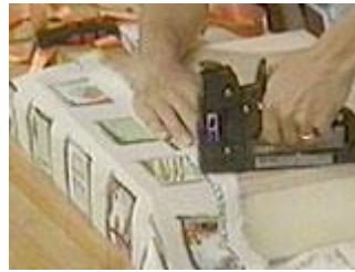
Staple the material on one side
