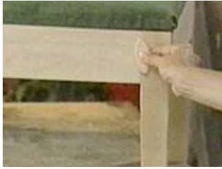
Where the biscuit fits in the joint
