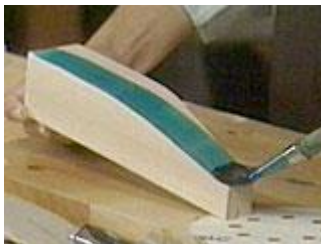
Brush on in one long stroke
