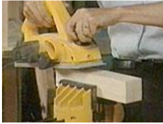
Begin planing against the grain on the thick end of the taper
