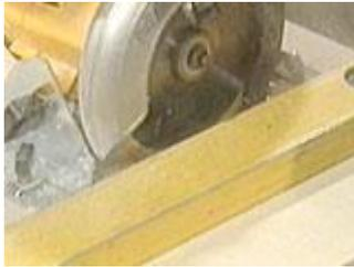
Make the cut using a straight edge
