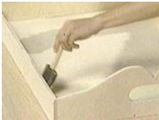
Apply the undercoat of paint first
