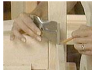
Set the brace on top of the apron to locate the slots
