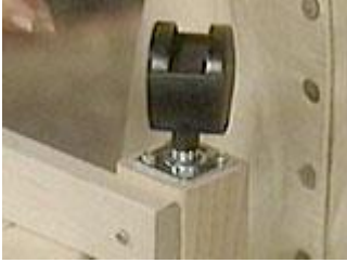
Attach the casters to the bottom of the legs
