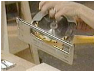
Set the depth of the blade to fit the brace
