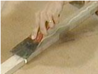
Apply glue on each side that touches another
