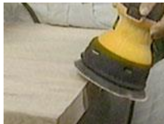
Soften the sharp edge with an orbital sander
