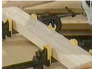
Place the boards in the pipe clamps and even up the ends
