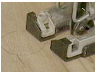
Cut out the shape with a scrolling blade in a jig saw
