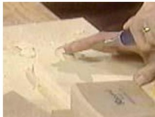
Chisel with the grain to finish
