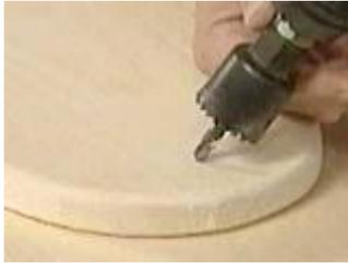
Use a hole saw to drill holes in either end
