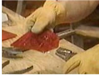
Breaking pliers have a wider mouth and are used to break the glass after scoring with the cutter
