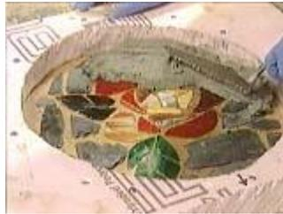
Place the mortar carefully in the mould over the glass
