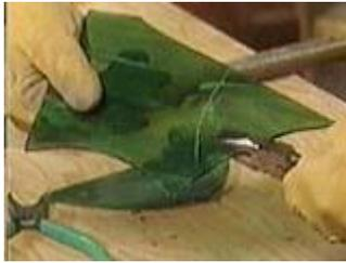
Use the breaking pliers to break along the line, down and away from the scored line
