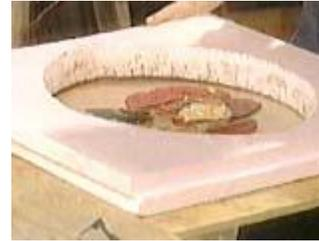
Place the design under the form on a small piece of plywood
