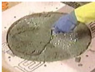
Fill the remaining space with concrete
