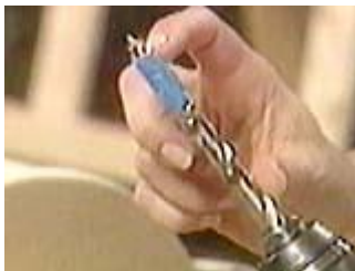
Using a brad point bit makes a clean hole for a plug
