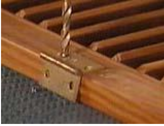
Drill off the heads of stripped screws
