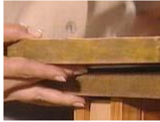
Place the larger base on top of the smaller one with the lazy Susan in between
