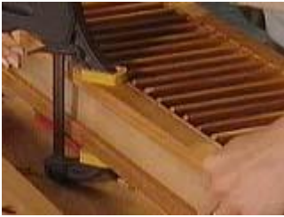
Clamp the 'sandwich' together and fasten with screws
