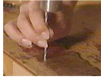
Use a hammer and nail to punch holes for the wires
