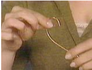
Form a hook with heavy copper wire
