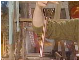
Use a fine copper or steel wire and don't allow the wire to touch the sides of the pipe
