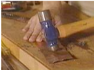
Use a ballpeen hammer to distress the copper
