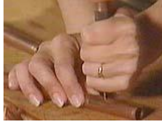
Use a compression punch to make a little dimple to prevent the drill bit from skating
