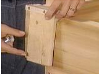
Make a jig for the holes out of a scrap piece of plywood
