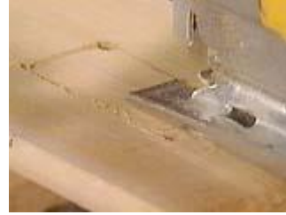
Cut out the hole for the leg...
