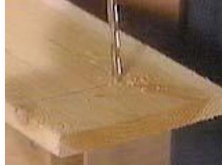
Drill a hole in each corner for the jig saw blade
