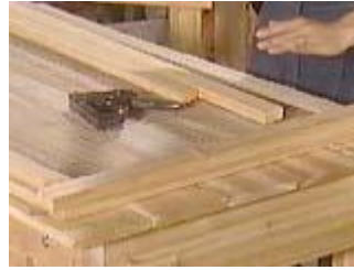
The second half of the frame is attached over the wire and front is screwed to the back
