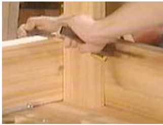
Clamp the leg in place before drilling
