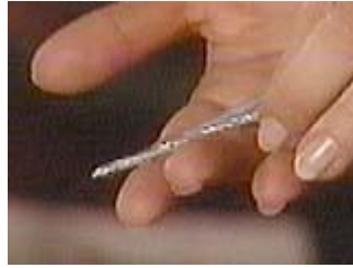
Use galvanized nails with a spiral shank
