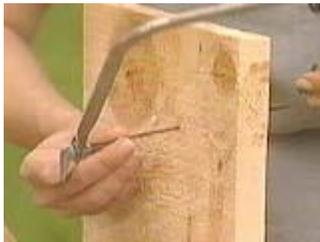
Pass the coping saw blade through the first hole, then reassemble the saw in position
