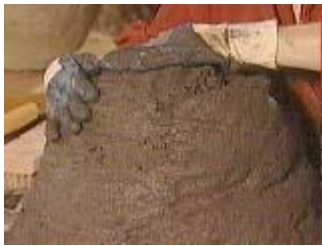
Press the bottom firmly onto the sides for a strong bond
