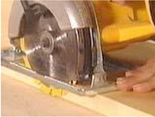
Adjust the depth of the saw blade to just cut into the surface of a scrap piece of wood
