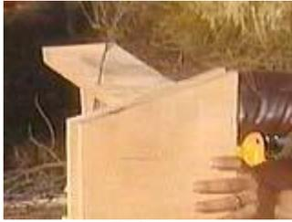
The side walls have a 15 degree angle for the roof line
