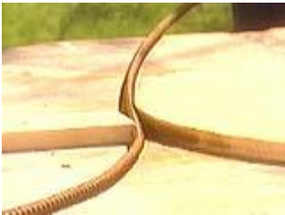
Turn it over to bend in the opposite direction
