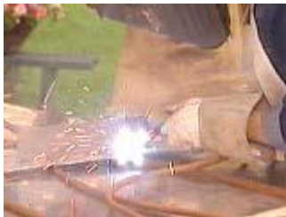
When the wire contacts the metal to be welded, the circuit is completed and the wire melts
