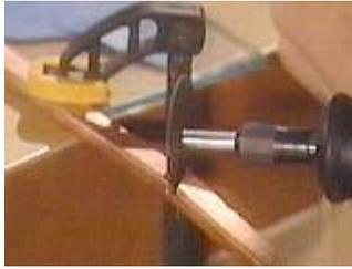
Be sure to hold the rotary cutter perpendicular to the metal
