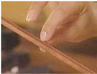
Metal with a channel used to frame the glass
