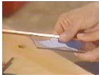
Use a scrap piece of glass inside the channel to prevent crushing when clamping
