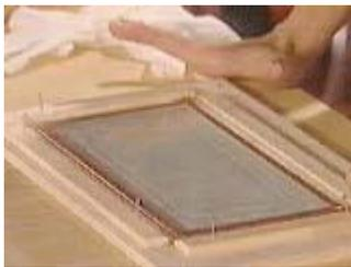
A wooden jig holds the copper frame in place while soldering
