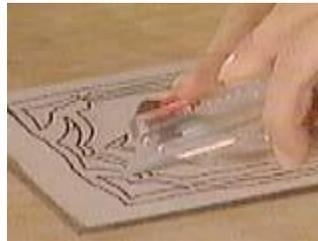
Cut along the pattern lines with a very sharp knife
