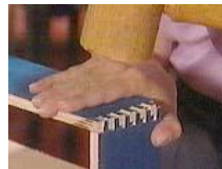
A good tight joint requires a mallet to tap the pieces together
