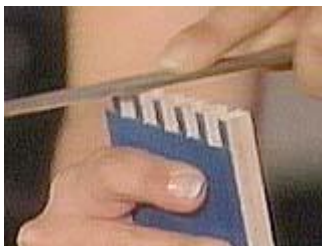
Use a file to clean up the joints
