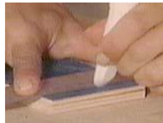
Transfer that size onto the wood and mark with a pencil or chalk
