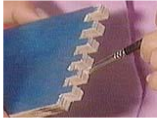
Brush glue on all the surfaces of every joint
