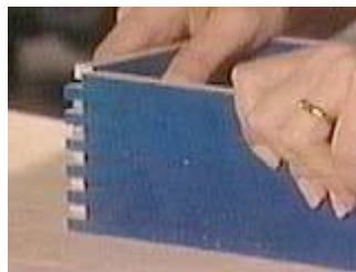
Dry fit the joints and choose the best fit
