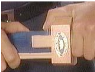
Draw the scribe along the end of each piece on both sides
