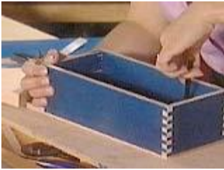
Place the box over a corner of spare plywood and trace the inside edge of the bottom dimension
