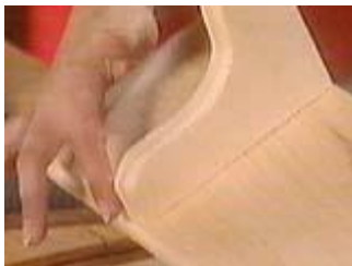
Use a scroll saw to cut brackets and a router to give the same edge as the shelf
