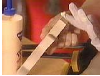
Use carpenters glue on both sides of the joint
