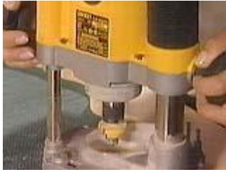
Use a router to give a decorative edge to the inside of the frame
