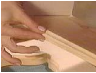
Rout the top and the bottom edge of the shelf
