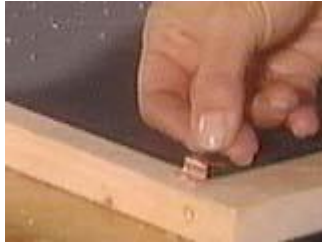
Bend it in a Z shape to fit over the mirror
