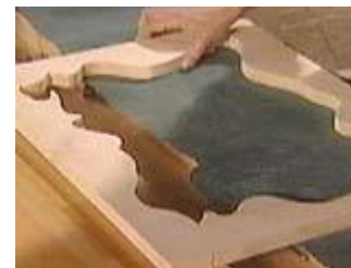
Place the frame on a non-skid mat for routing
