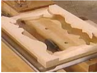
Place the top and bottom pieces on top of the sides and use a square for alignment
