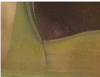
Close-up of a curved joint cut with a scroll saw
