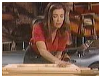
Screw the corners together from the top and the bottom for added strength
