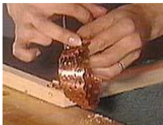
Attach pre-drilled copper plumber's tape to the back for hanging
