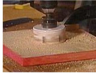
Cut a hole just deep enough to accept the clock mechanism
