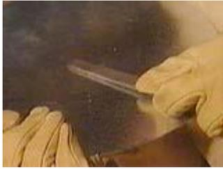
Use a file to clean up any burrs or sharp edges on the metal
