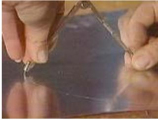
For a sheet metal face, scribe a cut line with a compass
