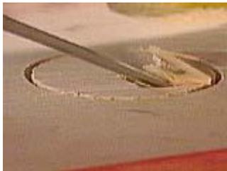
Chisel the wood out to the depth cut by the hole saw
