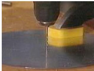
Enlarge the dimple first with a very small drill bit but don't go through
