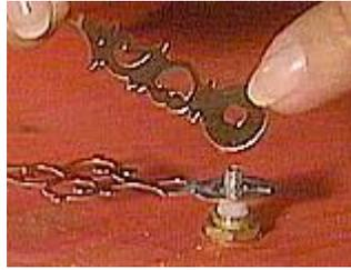
The minute hand is next and has a special slotted opening for the oval shaft
