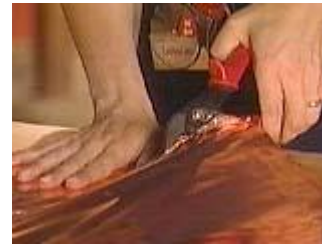
Cut the copper with the snips that work best for you
