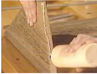
Apply glue to both sides of all the pieces that touch
