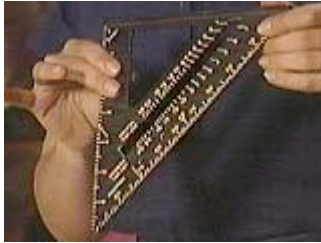
A speed square is a triangle with 90-degree and 45-degree sides
