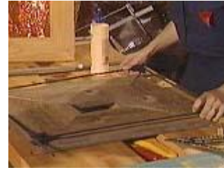
Place the frame clamp over the glued pieces and tighten it down
