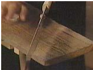
Use a Japanese style pull-saw to make the cuts
