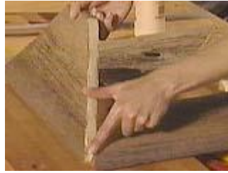
Use your finger to spread the glue around and remove any excess
