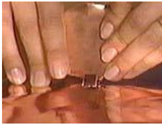
Pass it through the other slit and bend it up to secure it in place
