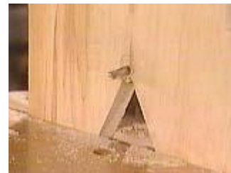
Drill a hole at the top of the 'V' to help prevent splitting
