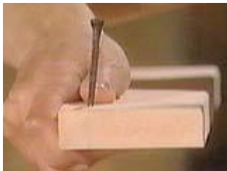
Orient the nail so that the narrowest dimension lines up with the grain
