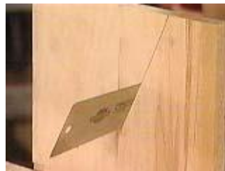
Cut out the v-notch creating the legs
