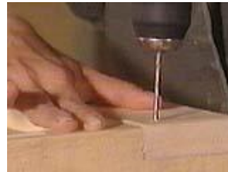
Drill for the nails
