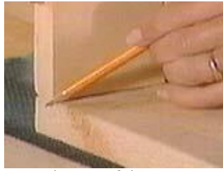
Trace the size of the supports on to the sides
