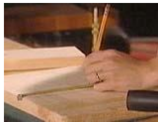
Find the height of the 'V' - not more than half the height of side
