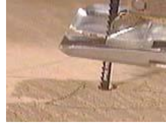
Put the jig saw scrolling blade through the hole
