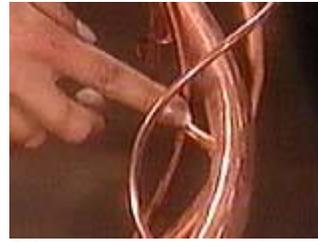
Drill holes in the larger pipe and insert smaller pipes as branches
