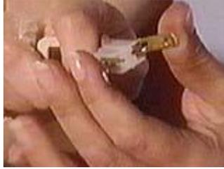
Squeeze the plug ends together puncturing the cord and making the connection
