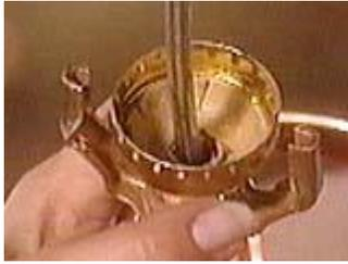
Slide the socket base over the end of the wire and the pipe
