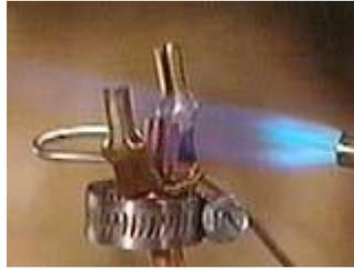
Always heat the pipe from one side and apply the solder from the other side
