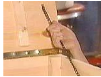
Choose a chain that is strong enough for the weight of the lid.
