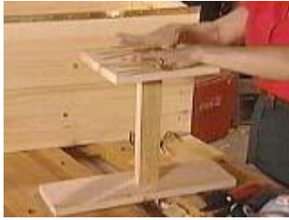
Make a jig to help hold the lid while attaching the hinge.
