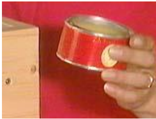
Use a food grade wax like bees wax to insure the finish is non toxic.
