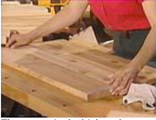
Three one inch thick cedar decking boards make the bottom of the chest.
