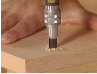
Drill the hole deep enough to allow for the wooden plug to go in.
