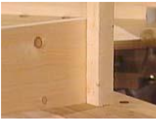
Attach the sides to the corner posts allowing room for the bottom boards.
