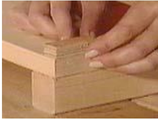
Make a jig to help locate the screws evenly.
