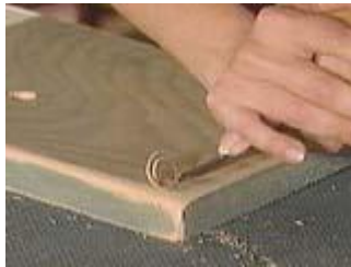
Carving using a v-groove carving tool
