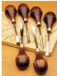
Set of carving tools for traditional carving ( you only really need the v-shaped one for this project)
