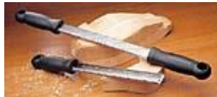
Wood rasp ( mine doesn't have a handle) - these are available at Lee Valley Tools
