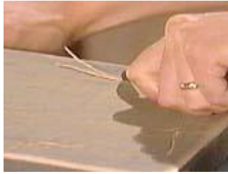
Carving using a chip carving knife
