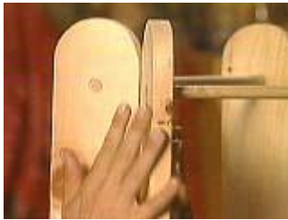
Completed arched ends with dowels.
