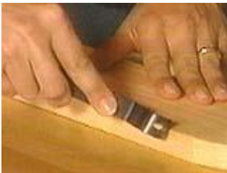
Use a cornering tool, sand paper or a plane to remove the sharp edge.
