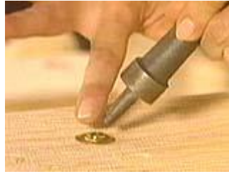
Place the grommet on the block or seat and then use the set to crimp.
