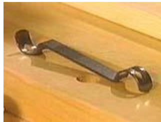
A cornering tool has two sizes of cutters for rounding sharp edges.
