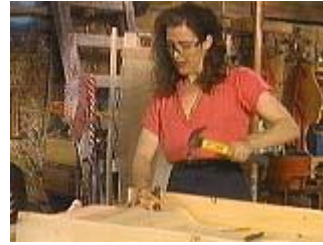
Crimp the grommet together using the set and the block or seat.
