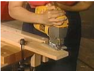
Cut the arched end using a jig saw.
