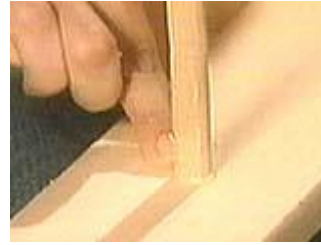
Clean up the excess glue.
