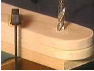
Drill a hole for the dowell in both sides using a backer board .
