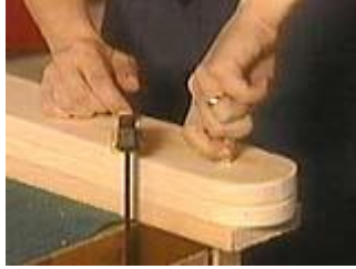
Roll a piece of sand paper to clean up the hole after drilling.
