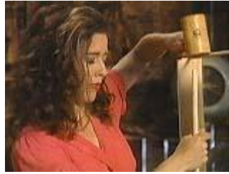
Pound the dowels into the hole using a wooden mallet.
