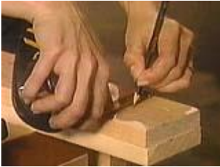
Mark the center of the board before using the compass to scribe an arc.
