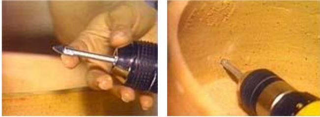
Drill a hole in the side of your container, somewhere near the bottom, using a glass/ceramic/tile bit. The hole should be the same diameter as the pump cord, so buy your drill bit accordingly.
