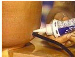
Next, put the pump back in your fountain container. Pull excess cord through the hole so most of the length is available to reach the AC outlet. Seal around the cord on both sides of the drilled hole using clear silicone sealant. Let it cure for 24 hours before moving it.
