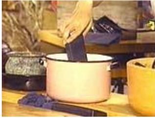
Fill a pail with water, drop the pump into it, and plug it in to make sure that your wiring is sound. This is a good time to experiment with the various attachments that come with your pump, to see what kind of flow pattern you want.
