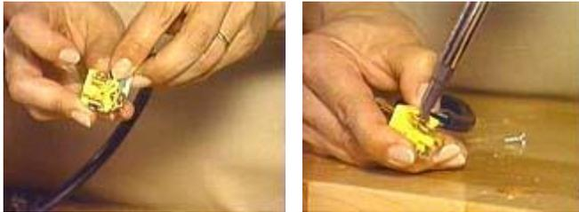
Now connect each of the three wires to the three screw terminals on the 3-prong replacement plug. The screws are different colours.
